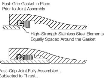
Proof-of-design tests have confirmed that the joints are capable of restraining deadend thrust of two or more times the rated working pressure, as applicable. These tests were accomplished with
