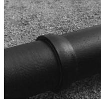
If the joint is to be deflected less than 2 1/4° for 20", 1 3/4° for 24", and 1° for 30", simply push the pipe spigot until it contacts the back of the socket and deflect. If the joint is to be deflected greater than these amounts, push the pipe spigot into the bell (while in straight alignment) only until the leading edge of the factory-applied yellow assembly stripe is even with the face of the bell. The desired deflection up to the maximum may then be set.
