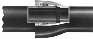
American Fast-Grip gaskets have been proven to be a superior field-adaptable method of restraining 4"-30" ductile iron pipe or fittings.
